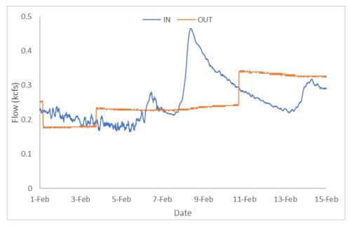
Figure 36. Hourly Flows In vs. Out (RO) (Fall Creek Tailrace)
